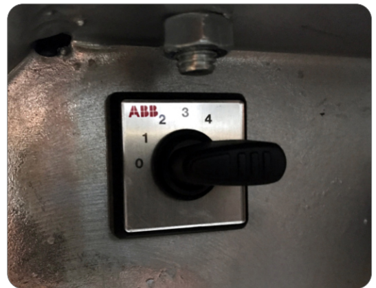
Speed adjustable up to 6 - 12 - 18 - 24m / hour
