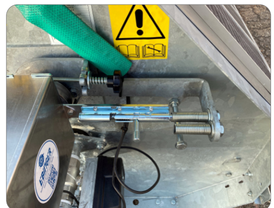
Electric motor for easy decoupling
